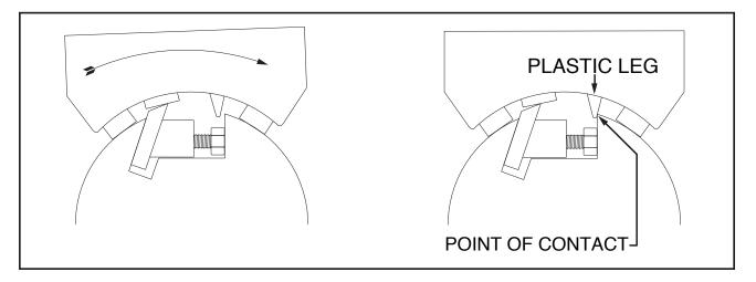
6. Hold the cutterhead with one hand and slide each jig until the indexing pin contacts the back edge of the gib slot. See Figure.
